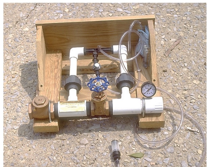
Figure 6. Fittings on the venturi injector, usually made of plastic, should be inspected for weathering.
