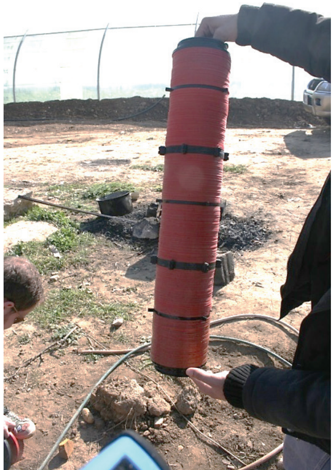
Figure 5. Sand that accumulates in disk filters can negatively impact filtering capacity and performance.
